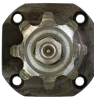
SPROCKET WEAR WITH DRAGO GATHERING CHAINS
